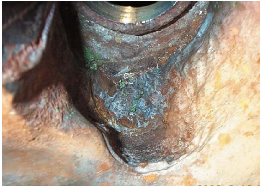
March 16: The unexpected “hole,” caused by boric acid, near a nozzle in the vessel head.
